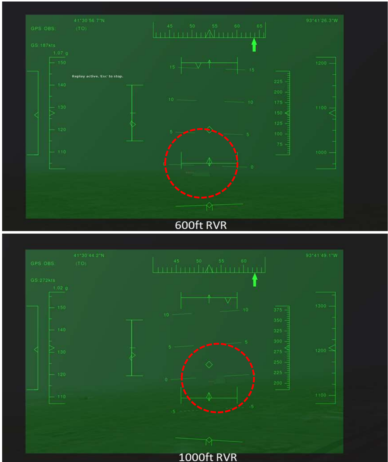
Figure 8. Simulated display in 1000 and 600 RVR (Red dotted circle indicates the runway environment). The runway is visible earlier in 1000 RVR (bottom figure) than in 600 RVR (top figure)
